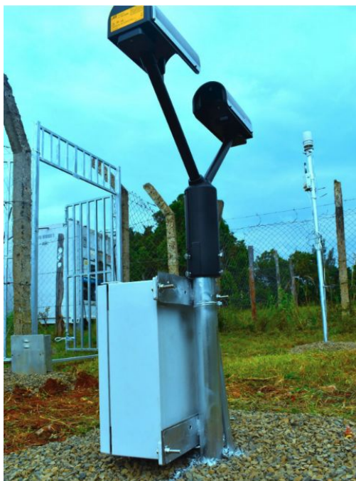
Image 2: A laser disdrometer deployed in Maseno University (Kisumu, Kenya)
